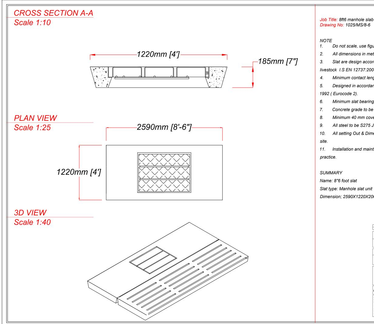
Do not scale, use figured dimensions only. All dimensions in metric and imperial units. Slat are design accordance floor slats for livestock I.S EN 12737:2004+A1:2007. Minimum contact length of slat on wall 100mm. Designed in accordance to BS8110 and EC2 Minimum slat bearing over wall 150mm. Concrete grade to be 50 N/mm<sup>2</sup> U.N.O. Minimum 40 mm cover to all steal. All steel to be S275 J0 to BS EN 10025. All setting Out & Dimensions to be checked on
